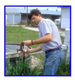
In the case of the nitrate test strips, these were held under a stream of water for one second and removed. The strip then made a color change within one minute if nitrate was present. The strips could indicate nitrate levels from 0-50 ppm.
